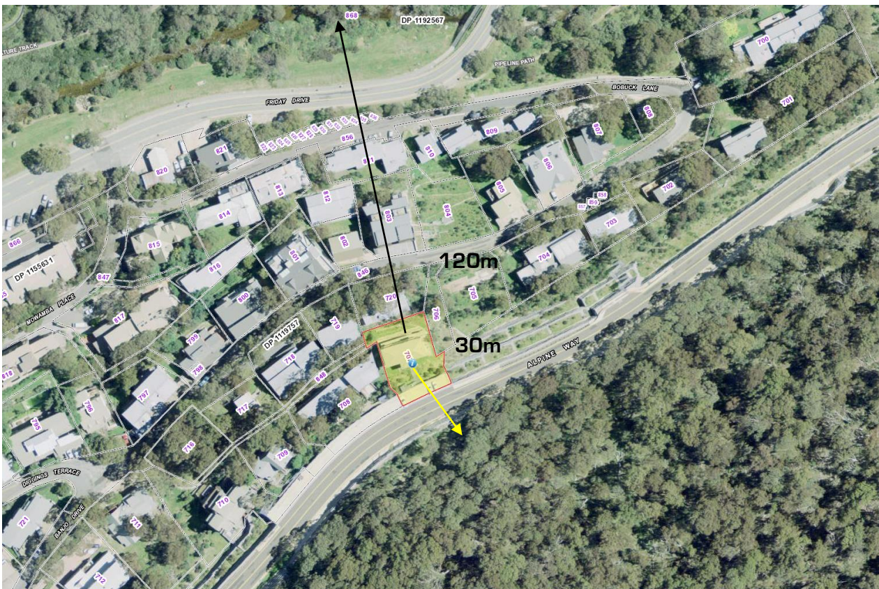
Figure 14: Aerial view demonstrating the distance to vegetation that would have the most influence in the event of a bushfire
